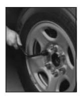
2. Use the wheel wrench to loosen all the wheel nuts.
